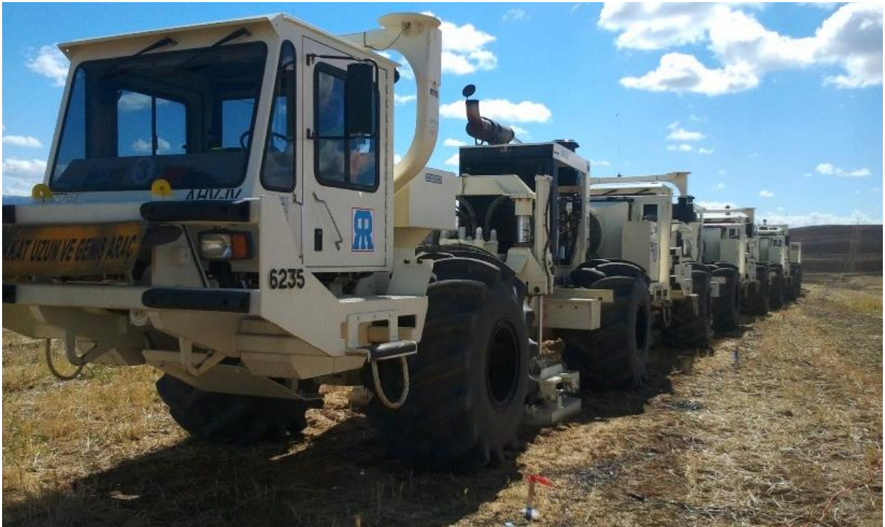
Figure 1. A view of the vibrator machine
